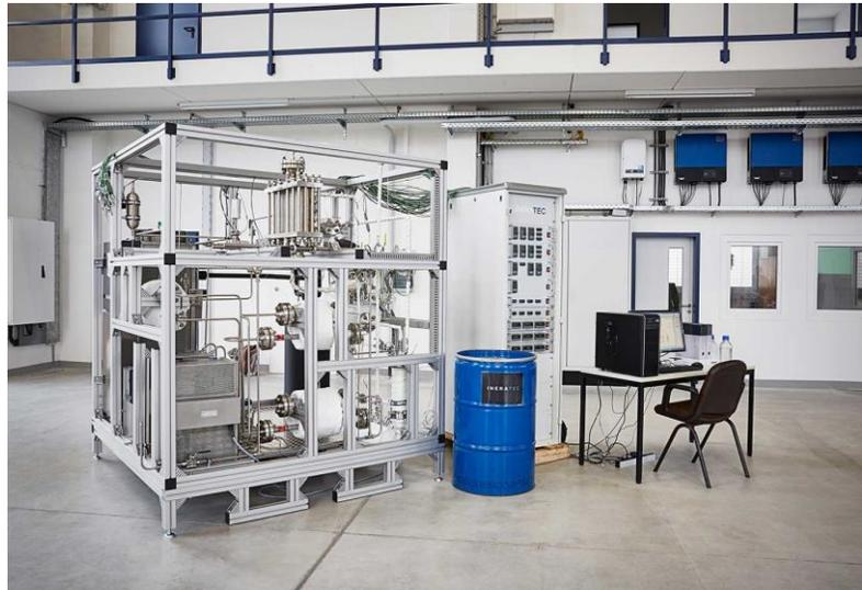
Figure 5. Mobile synthesis unit for a compact containerized CO<sub>2</sub> to fuel conversion plant [2].
