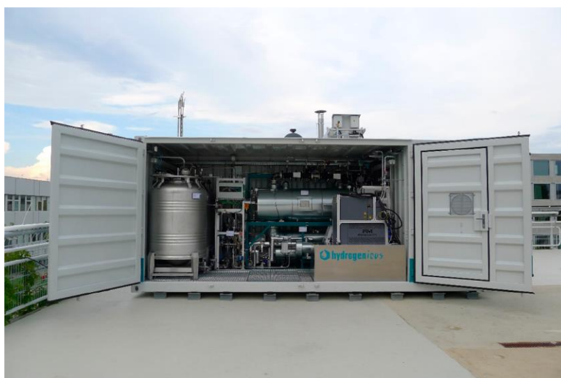
Figure – Top: Scheme for an off-grid liquid hydrogen organic carrier power supply where sufficient daytime sunlight runs the water electrolysis, re-hydrogenation and heat storage system LHS. Subsequently, the stored heat is used to run the de-hydrogenation unit RHS. Bottom: Commercial liquid hydrogen organic carrier demonstrator unit. Accounts of Chemical Research, 2017, 50, 74.
